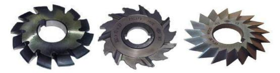
All of these cutters can be regrinding to standard size or specific modifications to suite profile. eg: Spline Profiles on Armature shafts
